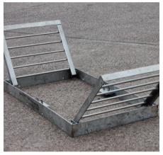
Steelway Bri-Grid SS is a stainless steel security / safety grid system designed to be retro-fitted into existing chambers that already have an access cover present. We can fabricate from sizes of 300 x 300mm up to 1000 x 2000mm in hinged sections. The Bri-Grid SS can also be fabricated in mild steel, galvanized to BSEN ISO1461.
